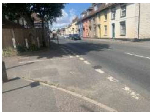
Figure 28: Footway parking reducing the footway width (Byssing Wood Road); wide junction radii prioritise turning vehicles and elongate pedestrian crossing (Canterbury Road)
