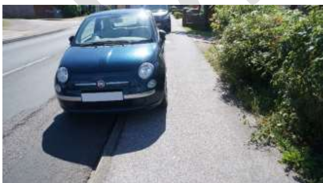
Figure 28: Footway parking reducing the footway width (Byssing Wood Road); wide junction radii prioritise turning vehicles and elongate pedestrian crossing (Canterbury Road)
