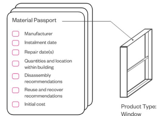
*Create material passports for products: This will improve the ability of disassembled elements to be reused. A material passport provides identification of materials, components and technical characteristics with guidance for deconstruction and applicability of re-use. In this way the building becomes a material bank for future use.*
