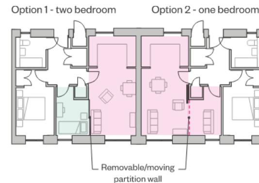
*Design for adaptation using a flexible floor plan e.g. one bed flat can be converted to a two bed flat or a one bed flat with space for home working. Working to a regular grid with removable partitions will allow adaptation as well as creating soft spots in the structure*
