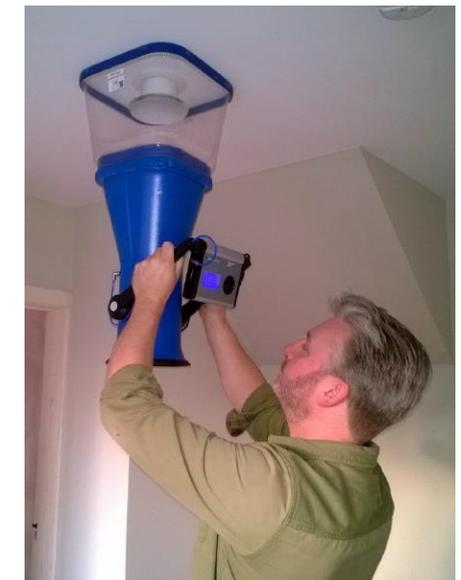
Flow rate measurement: image of MVHR system being commissioned (© Fourwalls)
