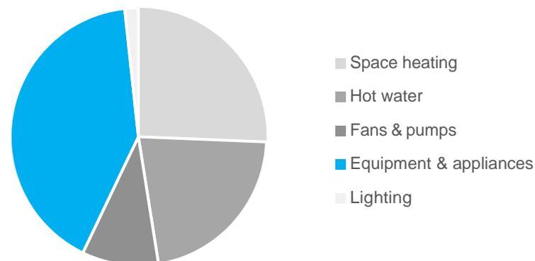
Electricity used by equipment and appliances is likely to be the largest end use of electricity in many net zero energy homes, so it is important to choose the most energy efficient appliances you can. Data based on energy modelling for a net zero energy new build home.
