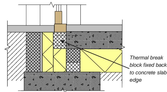
Sketch out key junctions and ensure there is a continuous line of insulation that runs around the building. Try to ensure the insulation depth does not reduce by more than a third around any junction, and ensure window and door frames are in line with insulation.
