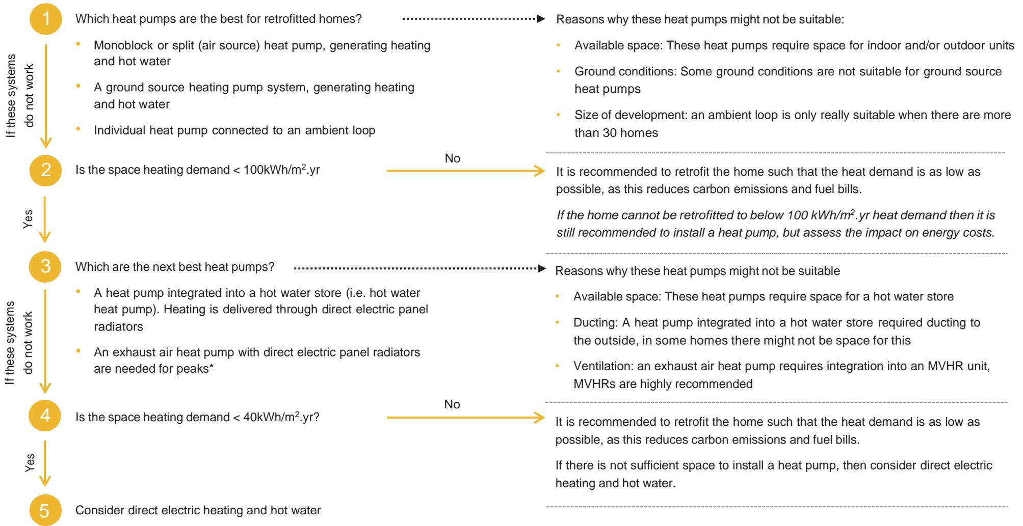
\*An exhaust air heat pump (compact unit) combined a heat pump and a MVHR. Some products can only meet the heat demand in smaller dwellings and/or this with a space heating <15kWh/m<sup>2</sup>.year,
