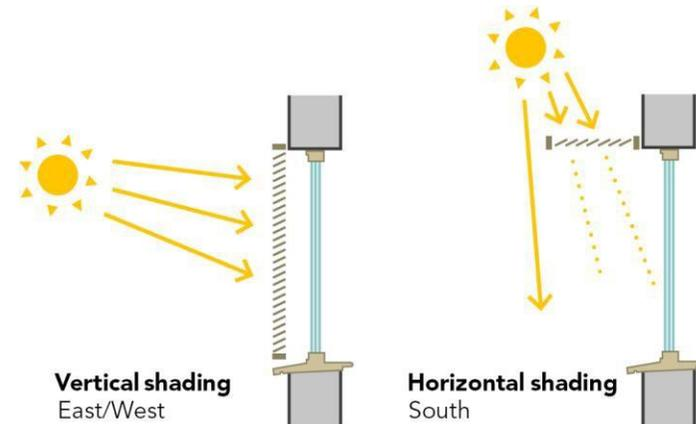
Provide horizontal shading on the south facade (e.g. brise-soleil or deep reveals) and vertical shading on the east or west facade (e.g. shutters). Design solar shading to allow useful solar gains in winter and block solar gains in summer.
