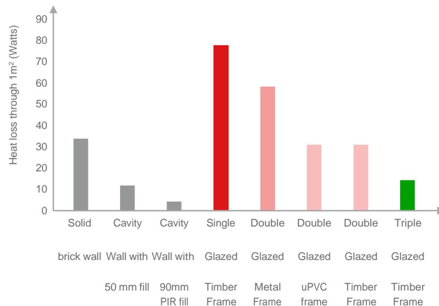
Heat loss through 1m<sup>2</sup> of various wall and window types (with 0°C external temperature)
