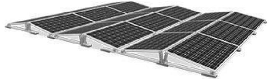
*East/West facing concertina type solar arrays are usually the best solution for the flat roofs of blocks of flats. They generate less energy per panel than rows of south facing panels, but achieve much higher panel densities as they do not require large gaps between the rows to avoid interrow shading.*
