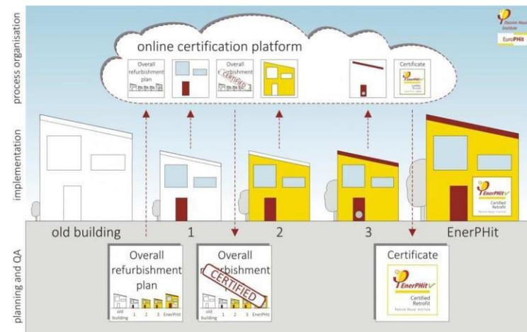
EnerPHit staged retrofit improvement plan process (© PHI)
