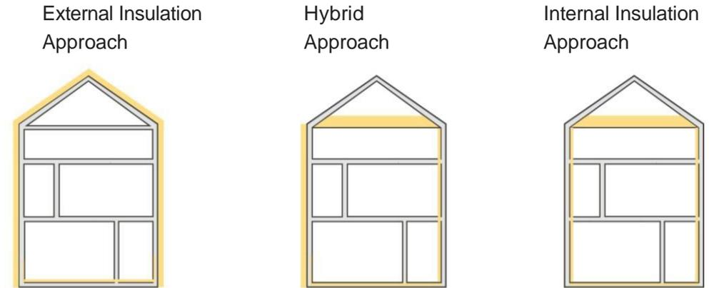
*In some circumstances, it may be beneficial to consider a hybrid approach e.g. internal insulation at the front to retain the architectural features of the front façade and external insulation at the rear. This maximises the insulation gains of using external insulation where it has less of a visual impact.*
