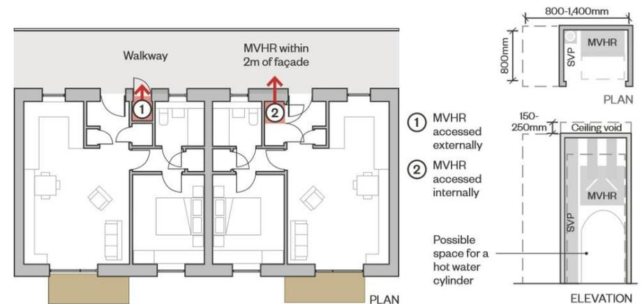
*MVHR systems are an effective way of providing ventilation to airtight homes.*
