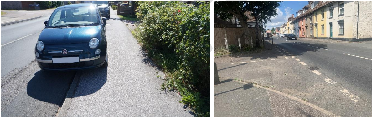
Figure 28: Footway parking reducing the footway width (Bysing Wood Road); wide junction radii prioritise turning vehicles and elongate pedestrian crossing (Canterbury Road)
