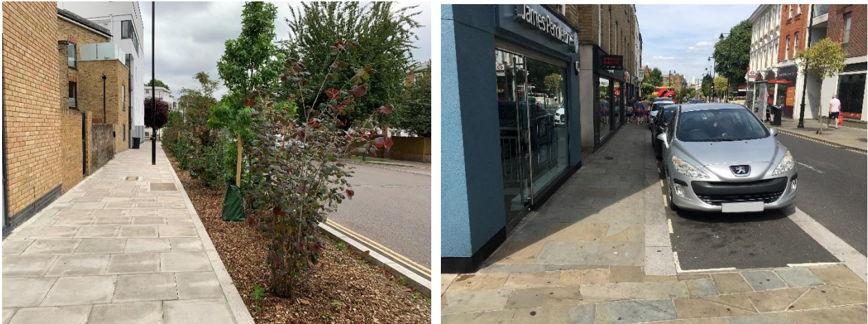
Figure 31: Example of clear footway space incorporating SUDs (Left – Crossway) and Recessed loading pads enable footway widening in constrained streetscapes (right – Clapham Old Town)
