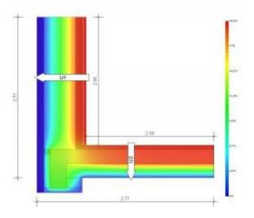
Consider commissioning thermal bridge modelling for particularly challenging junctions to inform your strategy. Small changes to the position and type of material used in construction can have a big affect on the heat flow, a model will help to show this.
