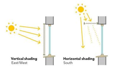
Provide horizontal shading on the south facade (e.g. brise-soleil or deep reveals) and vertical shading on the east or west façade (e.g. shutters). Design solar shading to allow useful solar gains in winter and block solar gains in summer.
