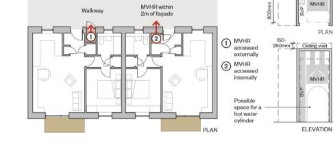
MVHR systems are an effective way of providing ventilation to airtight homes. The unit should be located within 2m of the façade
