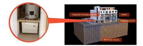
Diagram showing a passive ambient loop, with a small 'shoebox' style water source heat pump in each home connected to a ground array ( $\mathbb{C}$  Kensa)
