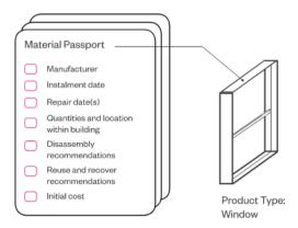
Create material passports for products: This will improve the ability of disassembled elements to be reused. A material passport provides identification of materials, components and technical characteristics with guidance for deconstruction and applicability of re-use. In this way the building becomes a material bank for future use.
