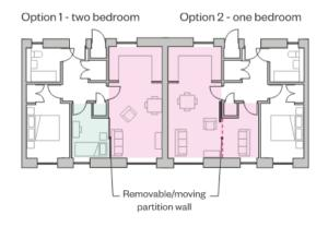
Design for adaptation using a flexible floor plan e.g. one bed flat can be converted to a two bed fat or a one bed fat with space for home working. Working to a regular grid with removable partitions will allow adaptation as well as creating soft spots in the structure
