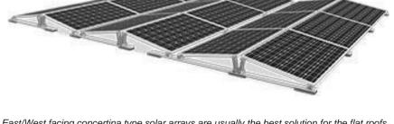
East/West facing concertina type solar arrays are usually the best solution for the flat roofs of blocks of flats. They generate less energy per panel than rows of south facing panels, but achieve much higher panel densities as they do not require large gaps between the rows to avoid interrow shading.
