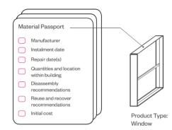
Create material passports for products: A material passport provides identification of materials, components and technical characteristics with guidance for deconstruction and applicability of re-use. In this way the building becomes a material bank for future use.
