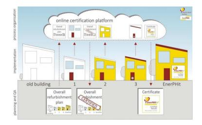
EnerPHit staged retrofit improvement plan process (© PHI)
