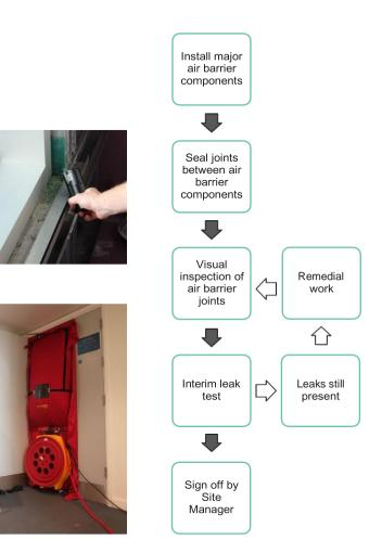
Recommended airtightness process: visual inspection, leak finding and interim air testing are all required before the final air test
