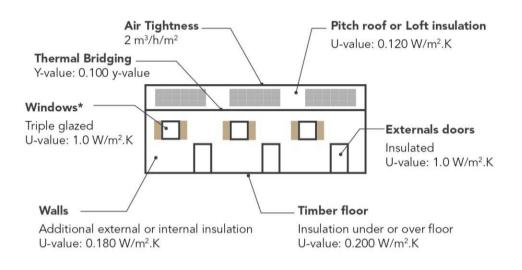
Recommended U-values to target net zero carbon for a constrained property.
